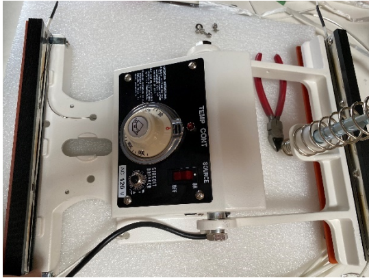
Figure 10. Loosen upper jaw from lower jaw
