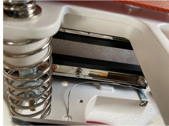
Figure 11. Loosen the screws found on the sealing jaws
