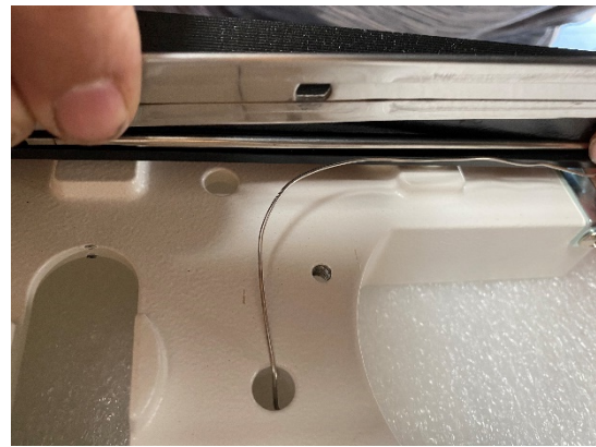
Figure 13. Install lower heater over the sensor
