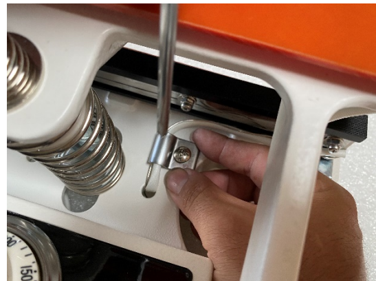
Figure 16. Replace lower bracket keeping lower heater in place.
