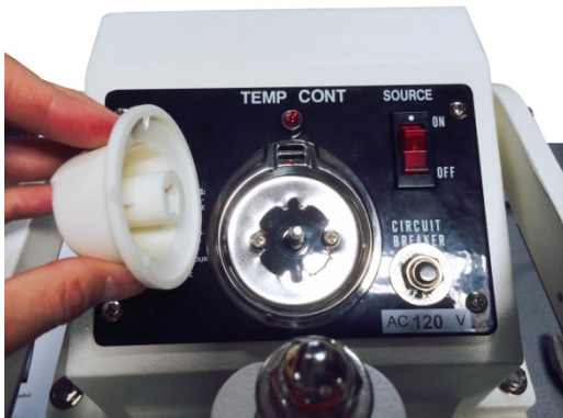
Figure 17. Remove thermostat cap.
