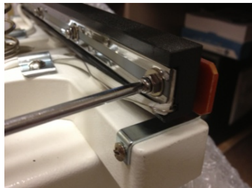
Figure 20. Unscrew heaters from bottom sealing jaw
