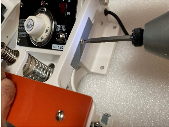
Figure 6. Remove the brackets holding the upper heater
