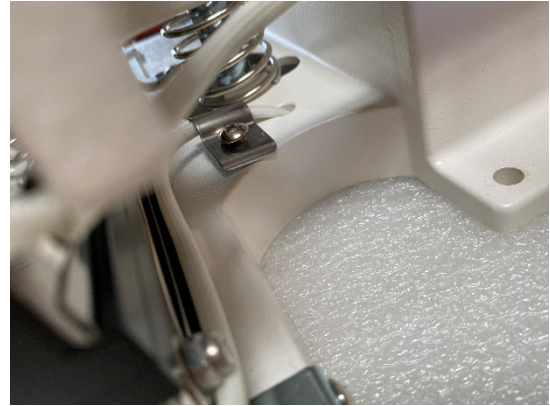
Figure 7. Remove the brackets holding the lower heater
