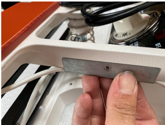
Figure 15. Replace upper bracket keeping upper heater in place
